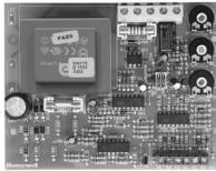
The interface board is a signal conditioner designed for the use in association a Honeywell modulation coil V7335A (Modureg). The purpose is to provide a linear conversion of a low DC voltage or current (produced by measure or control equipment) to a requested control current or voltage for the modulation coil (0-22 V-DC or 30-165 mA-DC).
